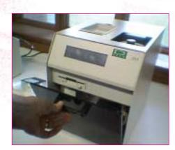
Sample type/handling: Automatic sampling from a 15 position carousel containing pre-diluted samples.
